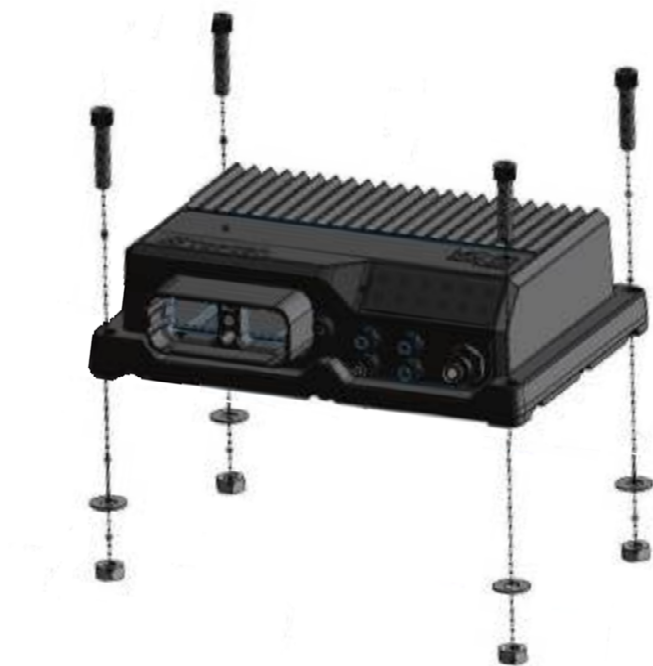
Figure 38: C-NavX3 Mounting
