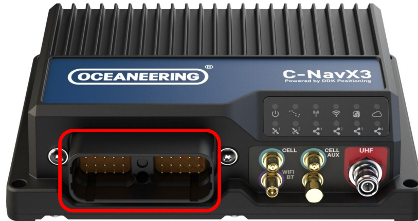
Figure 21: C-NavX3 Communications Ports
