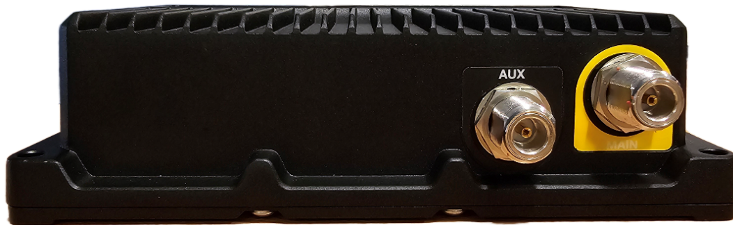
Figure 20: C-NavX3 GNSS RF Ports
